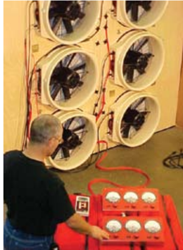
Retrotec's high-powered multi-door fan for large building testing.
